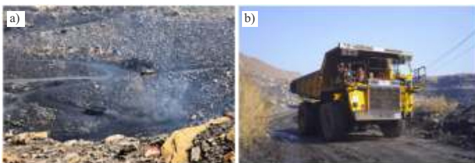
Fig 4. Dust generation a. before and b. after wet dust suppression and haul road stabilization
