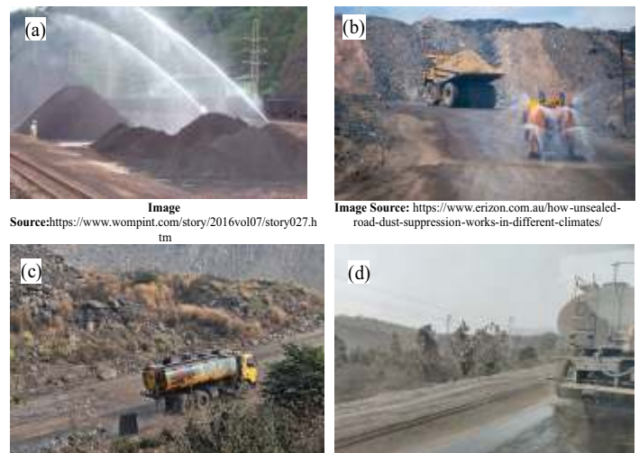
Fig. 3: Dust suppression using water
